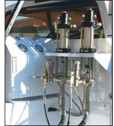
Multiple hydraulic-driven paint systems can be supplied. Easy access to hydraulic controls are standard.
