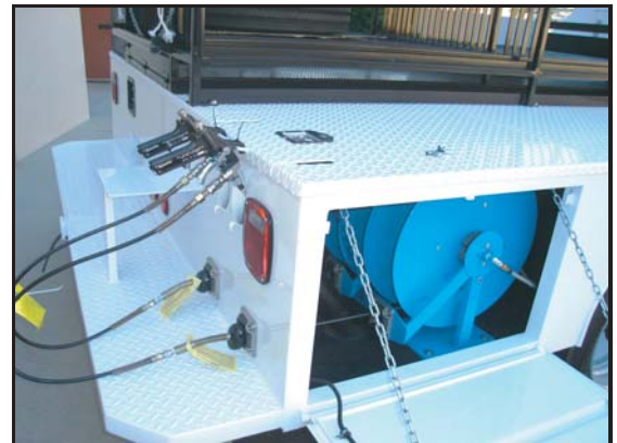
Hose reels mounted below deck with top and side doors for easy maintenance.
