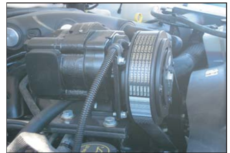
The electric clutch hydraulic system will vary in GPM for customer needs.
